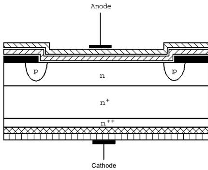
Fig. 3 Cross-sectional view of a Schottky diode
