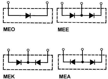
Fig. 16 Circuit diagrams for the available FRED modules
