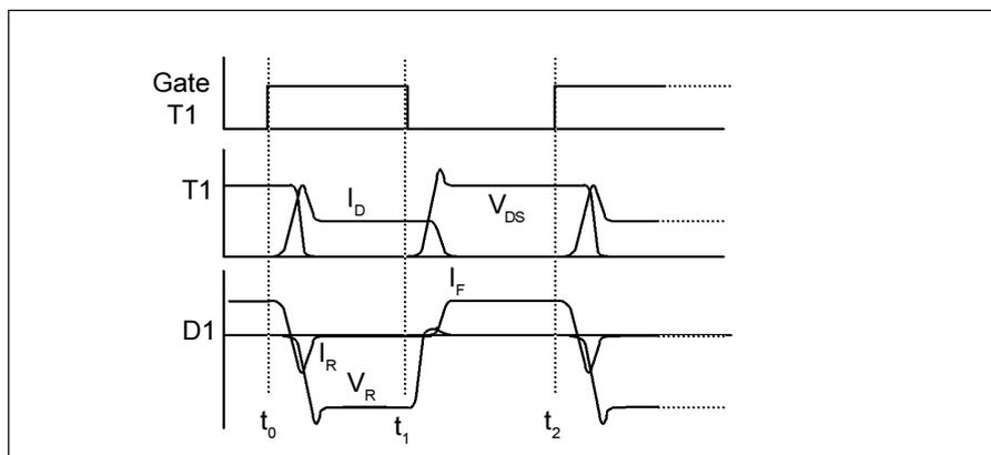
Fig. 7 Transistor gate signals, current and voltage waveforms along with the diode current and voltage waveforms for one switching cycle of the buck-converter shown in Fig. 6
