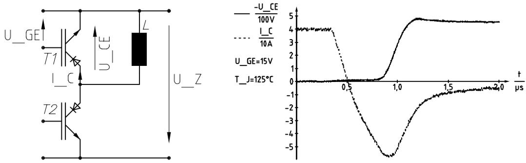
Figure 8: switching behaviour — turn off of the reverse blocking IGBT used as "controlled diode" in a chopper circuit
