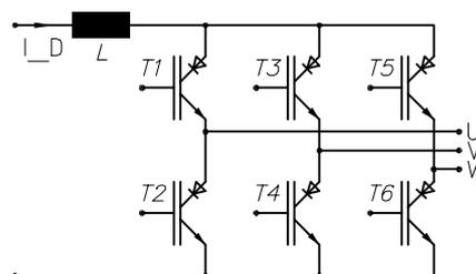
Figure 1: current source inverter
