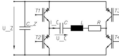
Figure 2: resonant circuit for induction heating
