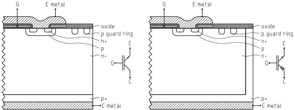
Figure 4: chip structure of and symbol used for NPT IGBT (left) and reverse blocking IGBT (right)
