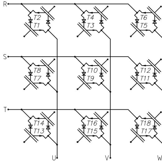
Figure 3: matrix converter with bidirectional switches
