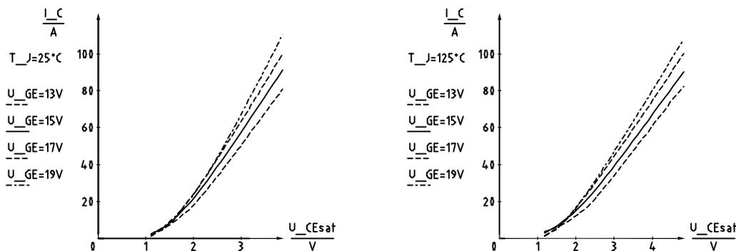
Figure 5: typical collector current versus saturation voltage at room temperature (left) and elevated temperature (right)
