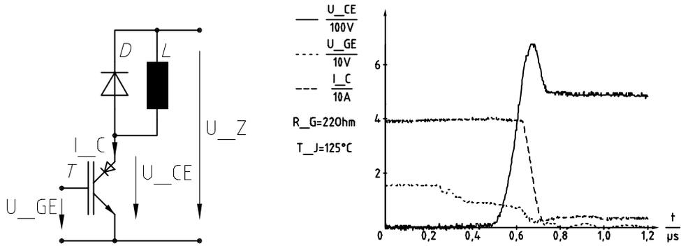
Figure 7: switching behaviour — turn off in hard switched chopper circuit
