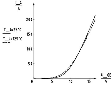
Figure 6: typical transfer characteristics at room temperature and elevated temperature
