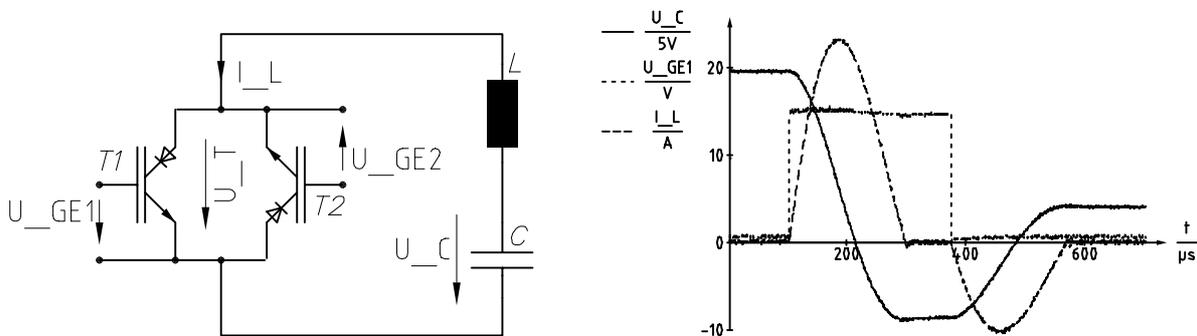
Figure 9: waveforms in a resonant circuit controlled by a bidirectional switch consisting of two reverse blocking IGBTs
