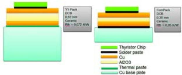
Figure 4: improved thermal construction (ComPack)
