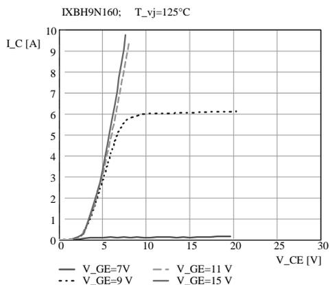
Figure 4b: output characteristics
