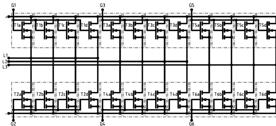
Figure 3: mechanical setup and circuit diagram of a power section with four paralleled trench MOSFET single switches in ISOPLUS 220<sup>TM</sup> package of IXUC160N075 type per switch
