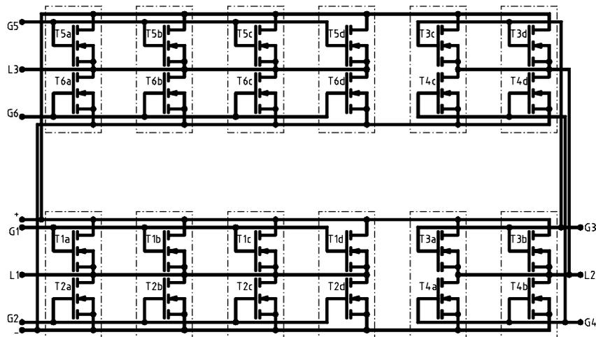
Figure 2: mechanical setup and circuit diagram of a power section with four paralleled trench MOSFET phaselegs in ISOPLUS i4™ package of FMM150-0075P type per phaseleg
