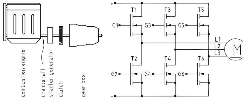
Figure 1: arrangement of and power section for starter generator
