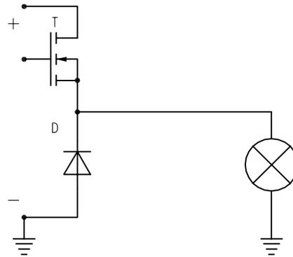
Figure 8: schematic of a load controller
