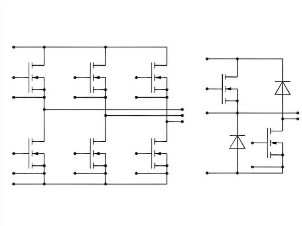
Figure 4: isolated module package  $40,4 \cdot 93mm^2$ ; sixpack and dual chopper topologies
