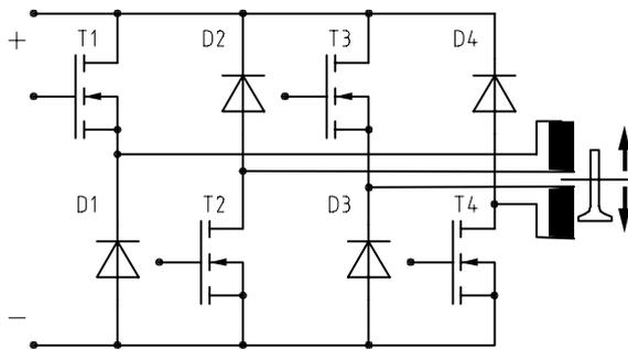
Figure 7: operational principle of a valve actuator
