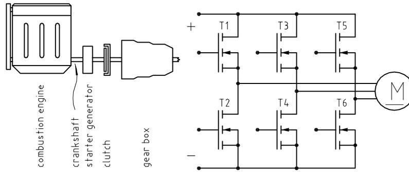
Figure 6: arrangement of and power section for starter generator
