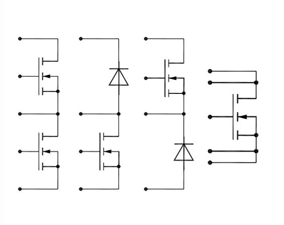
Figure 3: isolated ISOPLUS i4™ package  $19,9 \cdot 21mm^2$ ; phaseleg, chopper and single switch topologies
