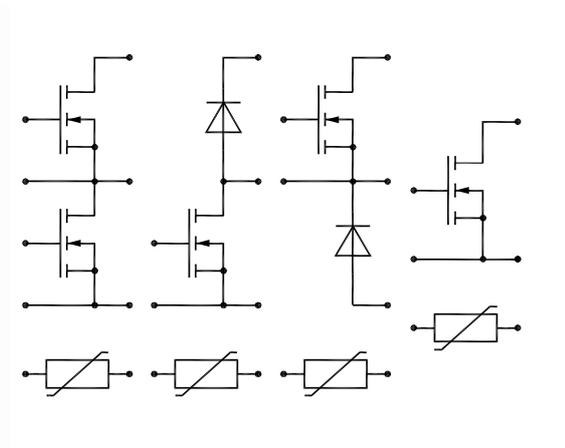
Figure 5: isolated module package  $62 \cdot 110mm^2$ ; phaseleg, chopper and single switch topologies
