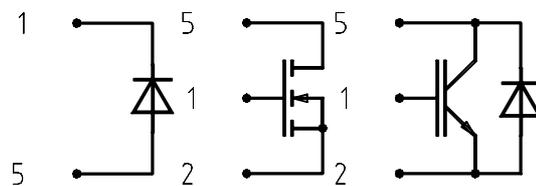
Figure 5: high voltage single switches with diode (left), MOSFET (center) or IGBT with diode (right)
