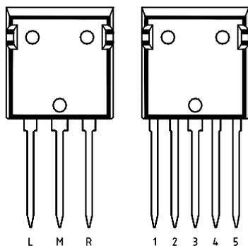
Figure 4: pinout of three pin (left) and five pin (right) version
