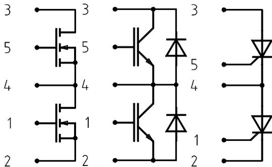
Figure 7: phaselegs with MOSFETs (left), IGBTs with diodes (center) or thyristors (right)
