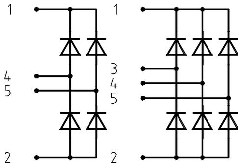
Figure 9: single (left) and three phase rectifier (right)
