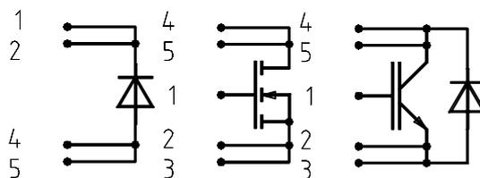
Figure 6: high current single switches with diode (left), MOSFET (center) or IGBT with diode (right)
