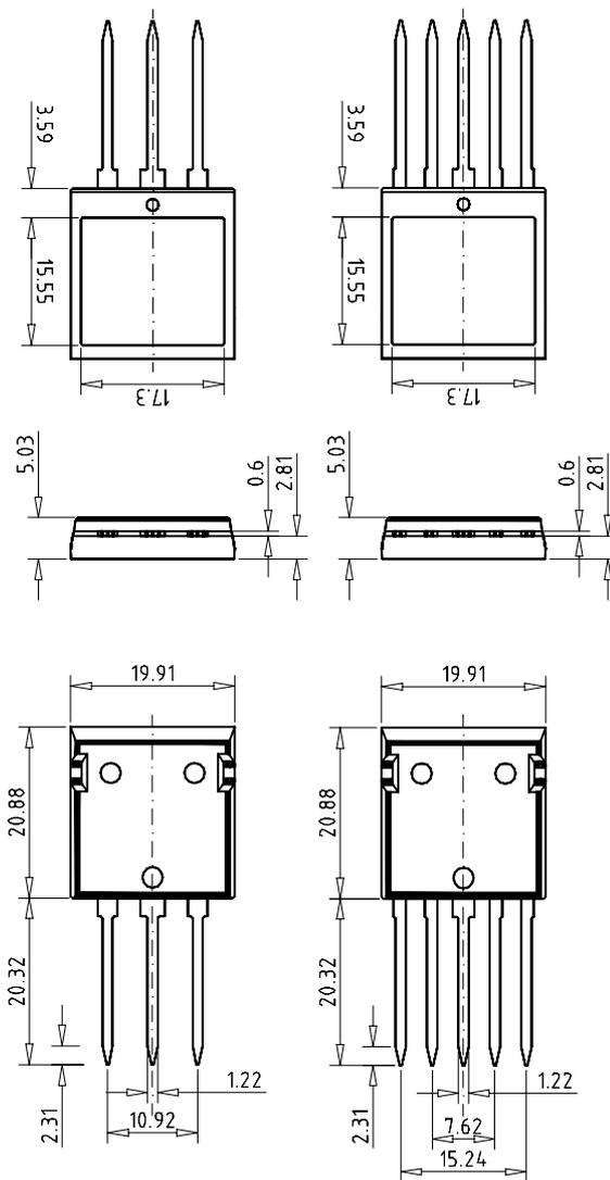
Figure 3: dimensional drawing of three pin (left) and five pin (right) version
