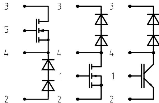
Figure 8: buck chopper with MOSFET (left), boost chopper with MOSFET (center) and IGBT (right), all with series connected free wheeling diodes
