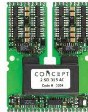
Driver stage for a gate current up to  $\pm 15A$  per channel, stabilized by large ceramic capacitors
