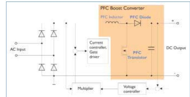
Figure 2. Simplified Power Factor Correction Circuit.
