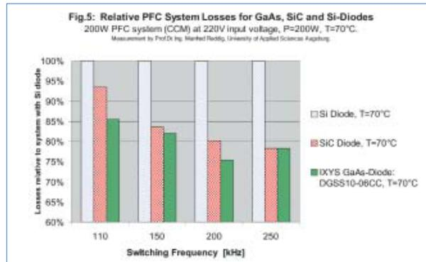
Figure 5. This graph compares the PFC system losses when using Si bipolar, GaAs and SiC diodes for different switching frequencies at 220V input voltage at 70°C. It can be seen that losses can be reduced by 15-25% when GaAs or SiC diodes are used.
