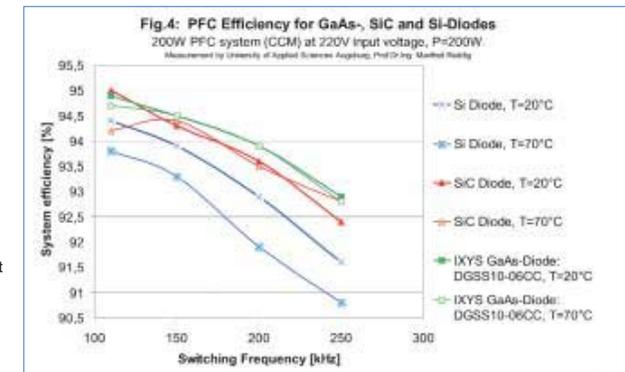
Figure 4. PFC efficiency for different diode types and temperatures vs. switching frequency at 220V input voltage.
