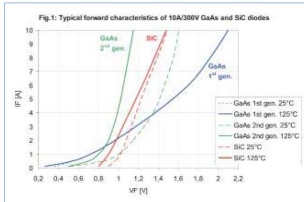
Figure 1. Typical forward characteristics of Gen.1 and Gen.2 GaAs and SiC Schottky diodes, 300V/10A types.
