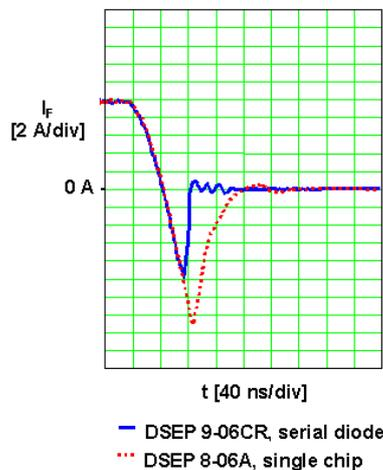
**Fig. 8:** Comparison of series connected diode to single chip type;  $I_F=10\text{ A}$ ,  $-di_F/dt=300\text{ A}/\mu\text{s}$ ,  $V_R=400\text{ V}$ ,  $T_J=150^\circ\text{C}$
