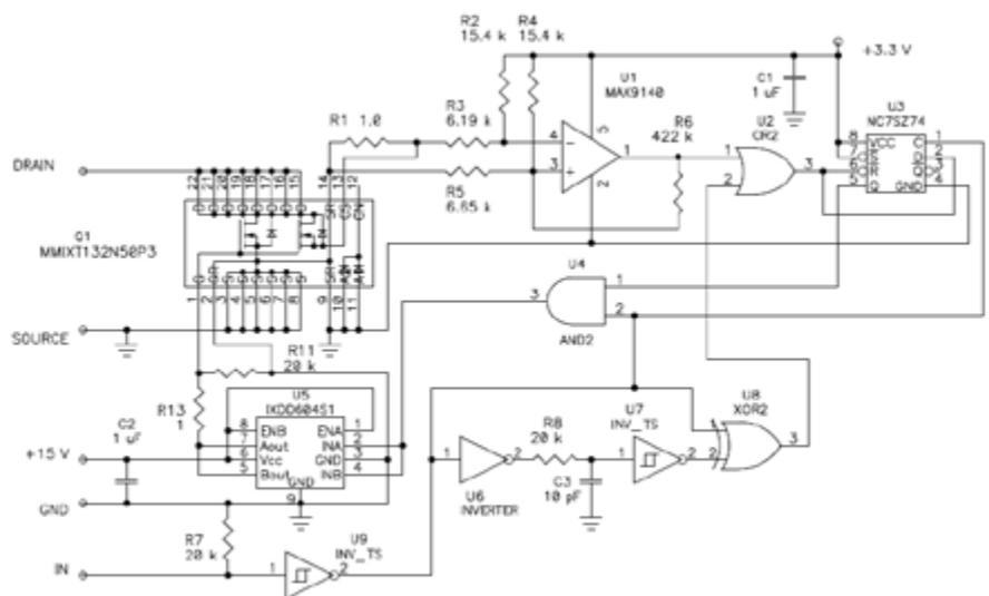
Figure 13: Positive Current Cycle-by-Cycle Overcurrent Monitoring System
