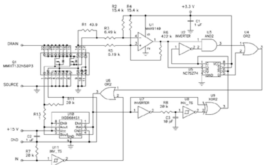
Figure 14: Negative Current (Body Diode Current) Monitoring System
