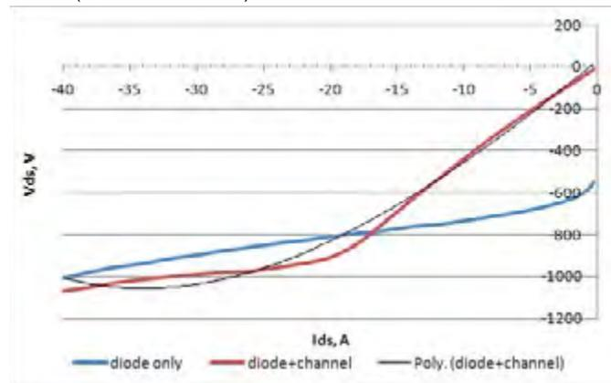
Figure 9:  $V_{DS}$  vs.  $I_{DS}$  at high negative currents
