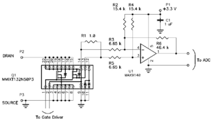
Figure 12: Positive Current Mirror Current Measurement Circuit
