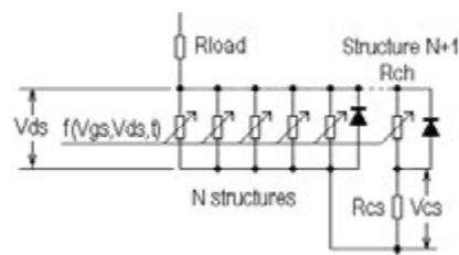
Figure 2: Current Mirror Schematic Diagram
