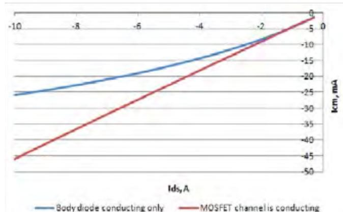
Figure 8:  $I_{CM}$  vs. Negative  $I_{DS}$  with MOSFET in ON and OFF States
