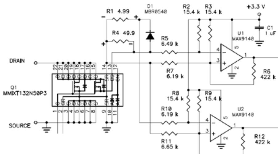
Figure 15: Separating Current Sense Resistors with Diode
