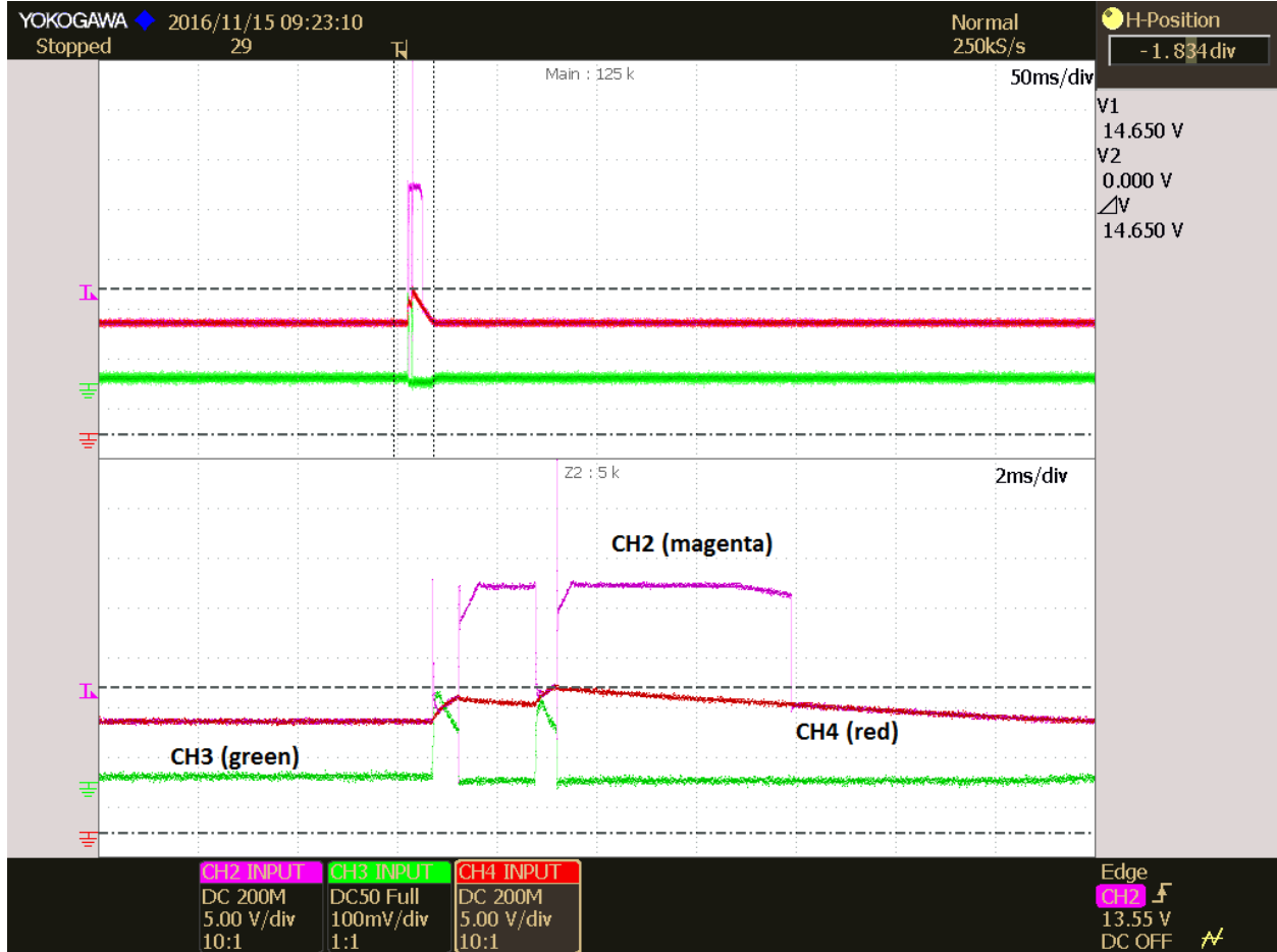
Figure 11: Dynamic Error in OV, if Minimum On-time set by MCU is too long
