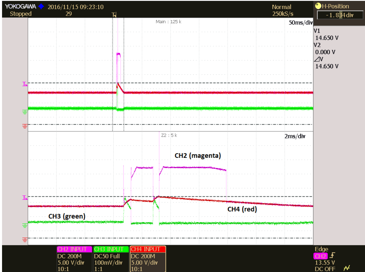
Figure 10: Operation with the Input Voltage Short Spike
