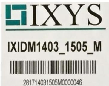
Phase-leg IGBT Module Marking
